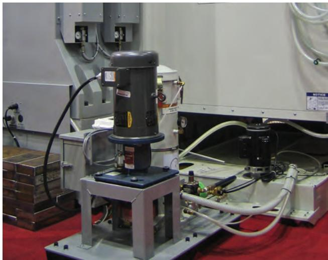
The seal-less design of Hydra-Cell pumps provides many advantages over other machine tool coolant pumps including the ability to handle abrasive fines and large-diameter particles.
