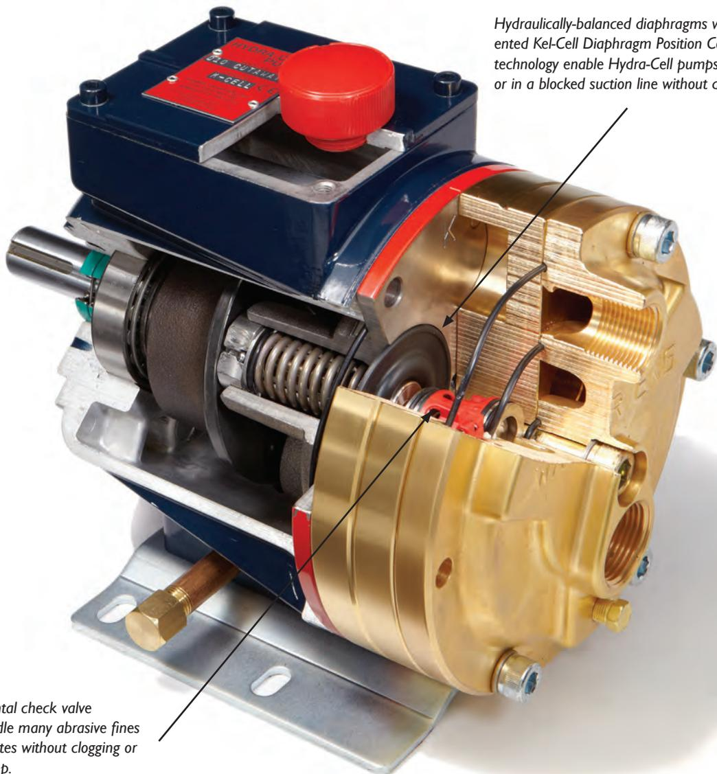
*Hydraulically-balanced diaphragms with patented Kel-Cell Diaphragm Position Control (DPC) technology enable Hydra-Cell pumps to run dry or in a blocked suction line without damage.*
