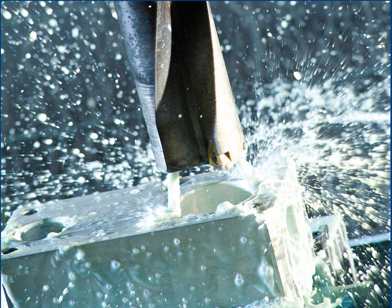
**Machine Tool Coolant**
