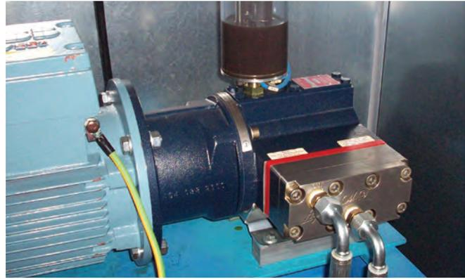
Compared to other pumps, Hydra-Cell requires minimal maintenance for polyurethane processors. Hydra-Cell has no mechanical seals, cups or packing that leak or need to be replaced and no internal gears to wear.
