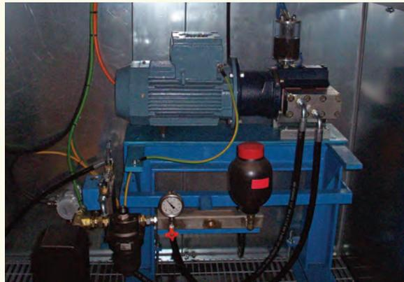
Pumping blowing agents requires a refrigeration unit. Significant capital savings are realized because space-saving Hydra-Cell pumps can be housed in a smaller refrigeration unit compared to pump types with the same flow and pressure ratings.
