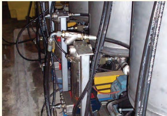
Injection of a proprietary catalyst into a high-volume polyurethane system. Where high flow is needed, Hydra-Cell pump models have maximum flow rates up to 66 gpm.
