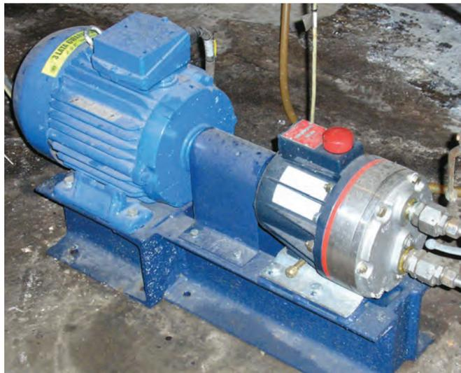
Hydra-Cell pumps also offer metering capability for OSB production as shown in the delivery of waxes and resins.
