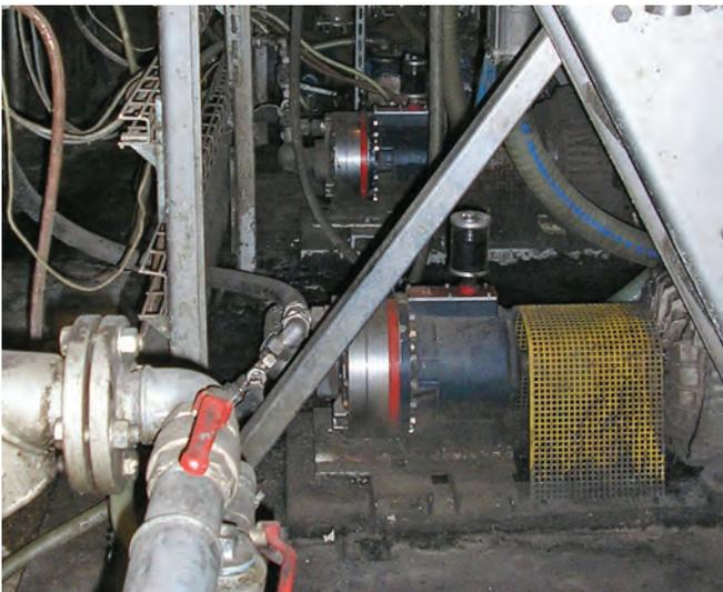
Hydra-Cell pumps provide high-pressure spraying of glue required for manufacturing plywood.
