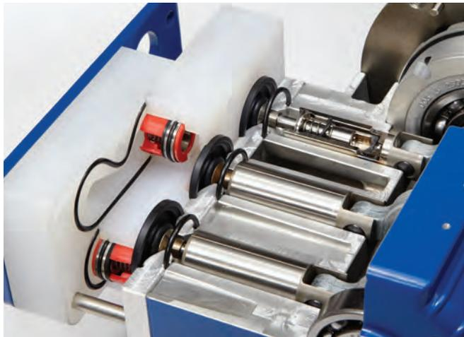
The multiple-diaphragm liquid head of Hydra-Cell also allows a less expensive, energy-saving motor to be used.
