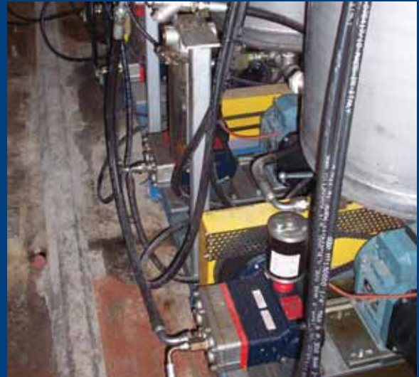
Injection of a proprietary catalyst into a high-volume polyurethane system. Hydra-Cell can provide precise metering and dosing when low flow rates are required.
